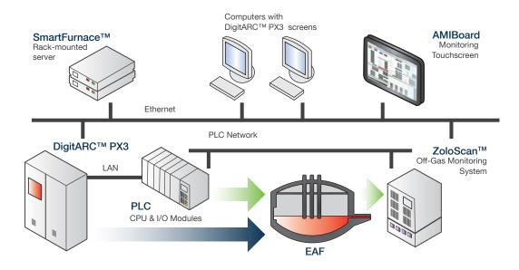
AMI's SmartFurnace™ System utilizes several individual modules to adapt and optimize every aspect of the furnace operation. The open architecture allows EAF is operate with the best performance at all times according the specific needs of the customer.
